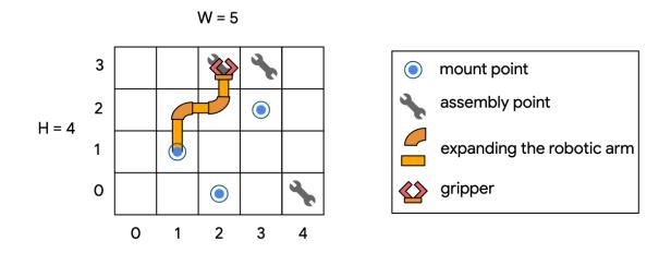
Robotic arms can move the gripper and expand to one of the four neighbouring cells (up/down/right/left - *not* diagonally). Robotic arms can **expand** as far as needed inside the assembly workspace. Robotic arms can also **retract**, moving the gripper back into the previous cell occupied by the robotic arm, and toward the direction of the mount point. Robotic arms can also **wait** in place without moving (for example, waiting to expand until a neighboring cell becomes free).
