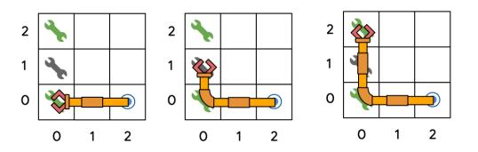
**Figure.** The green assembly points need to be visited for task 0. Even though the gripper also visits the assembly point at [0, 1], this does not count toward completing task 1, because the arm was working on task 0 when the gripper was in [0, 1].
